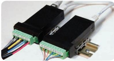
The menu items for these modules do not appear until the module is connected, simplifying the basic menu. Relay and digital I/O modules are shown above with optional DIN rail mounting kit, P/N PDA1002.
